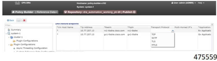
Figure 56: DRA Inbound Endpoints - Example Configuration
