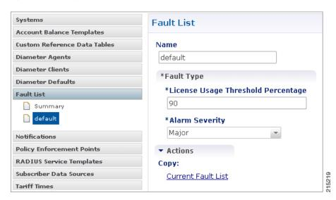
Step 4 Choose a Name for the Fault List. Currently, only License Usage Threshold Percentage fault type is supported. The Alarm Severity can be configured to be one of Critical, Major, Minor or Warning.
