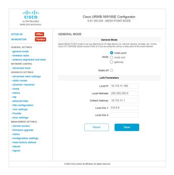
The **General Mode** has the operational mode controls. Devices capable of operating in a mesh radio network are shipped in **mesh point** mode.
