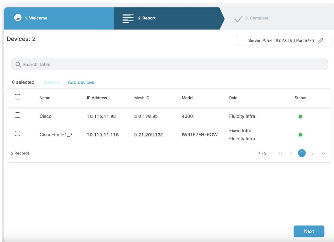
The screenshot shows the 'Report' step of the IW Monitor setup process. The interface has a top navigation bar with three steps: '1. Welcome', '2. Report' (which is the active step), and '3. Complete'. A sub-header 'Devices: 2' is displayed above a table. A status bar at the top right shows 'Server IP: 64.103.77.16 | Port 8443'. A search bar labeled 'Search Table' is present. The table lists two devices:
