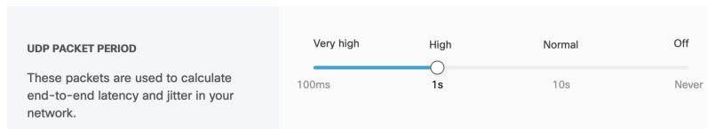
b) To disable the UDP packet transmission, click-and-drag the **UDP PACKET PERIOD** slider to **Off**.
