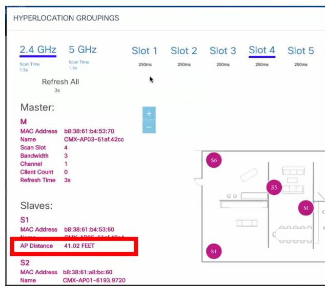
Observe that each slot has an allocated time which is listed below the slot. There are also two frequency bands, 2.4 and 5 GHz, each with scan times. Scan time is the total time allocated to scan every slot of a band at least once. Since there are two such bands, 2.4 and 5 GHz, the total Refresh time is the sum of these two, and is the time taken to scan all slots of all bands.
