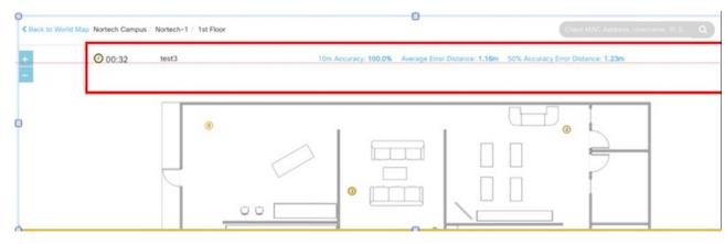
The test results displayed indicate that for 100% of the time, Cisco CMX locates the client within this many meters from where the client is actually located.
