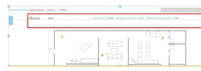
Step 13 Click View accuracy test report  $\bigcirc$  icon on the top-right corner of the window to view the list of accuracy tests that you performed. This report enables you to restart a test, download the latest log or all logs, or email the test results.
