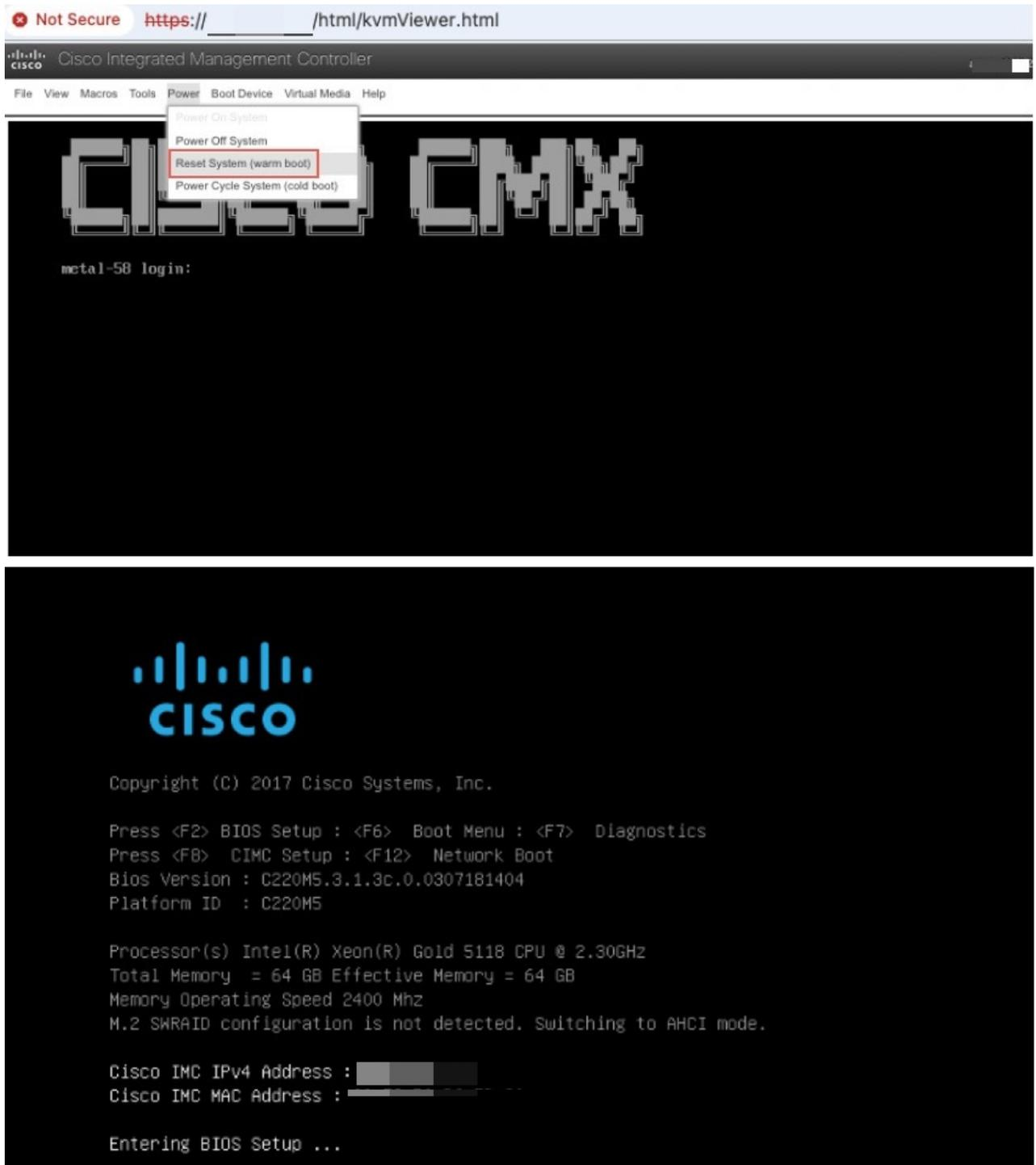
**Step 2** To enter into BIOS setup, press F2.
