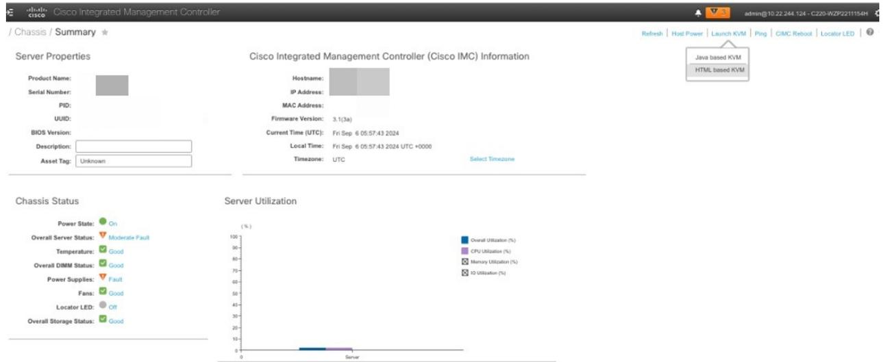
**Step 13** Click the link displayed to accept the certificate and load the KVM client application.
