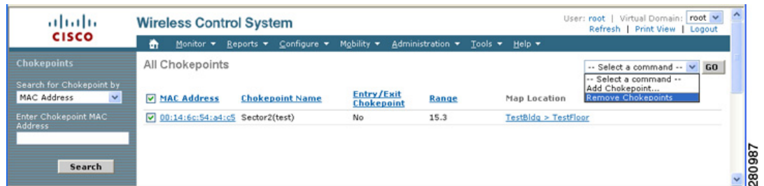
Figure 7-12 Removing a Chokepoint
