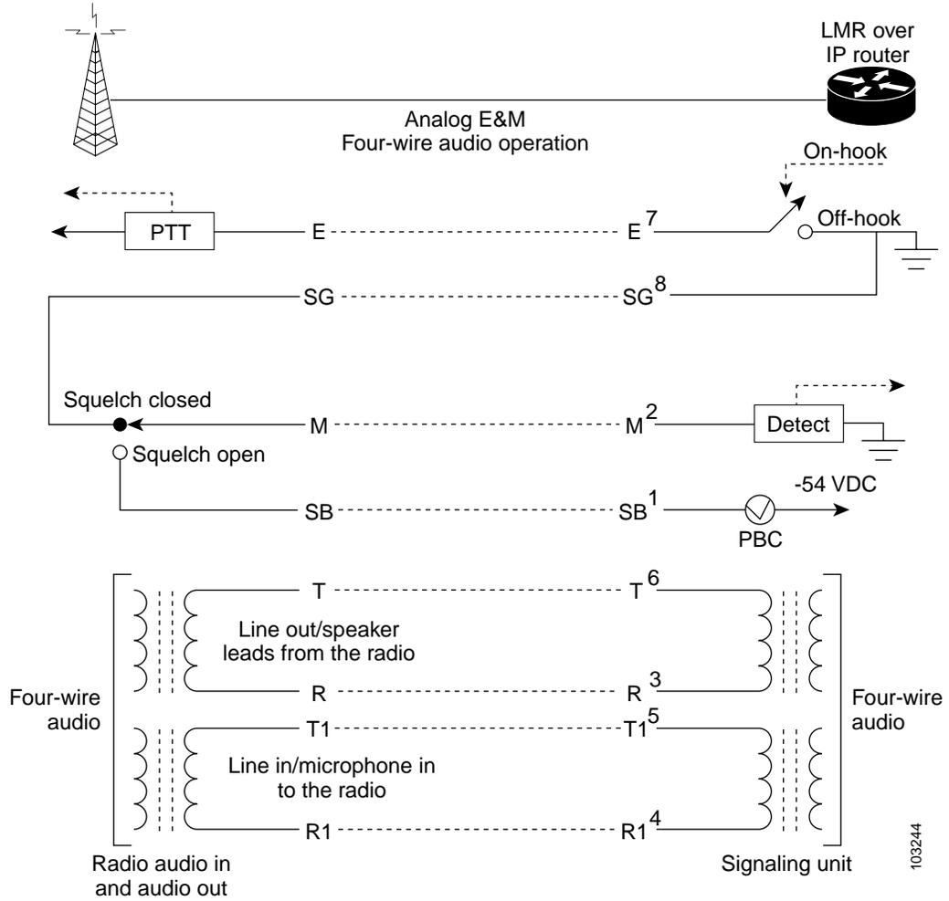
Figure 3-5 E&M Type V Interface Model
