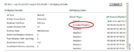
Because many nodes might be attempting to join or rejoin the network after an expected or unexpected event, a hold-off time of 16 minutes is implemented, which means that no nodes are exclusion-listed during this period of time after system initialization.
