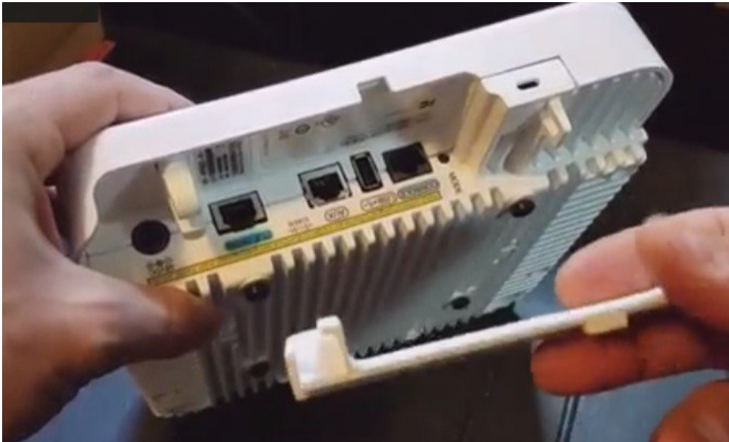
Figure 4: Example of a 3D printed cover installed
