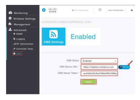
Tip Click the **Test Link** button to verify connectivity from Primary AP to CMX Cloud Site using the configured information.
