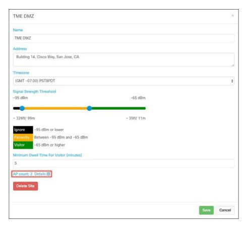
**Step 7** The window will expand and **Add new AP** field will be displayed. Enter the Base MAC Address of the Access point and click **Add**. When finished with adding Base MAC of AP to the sites, click on the **Save**.
