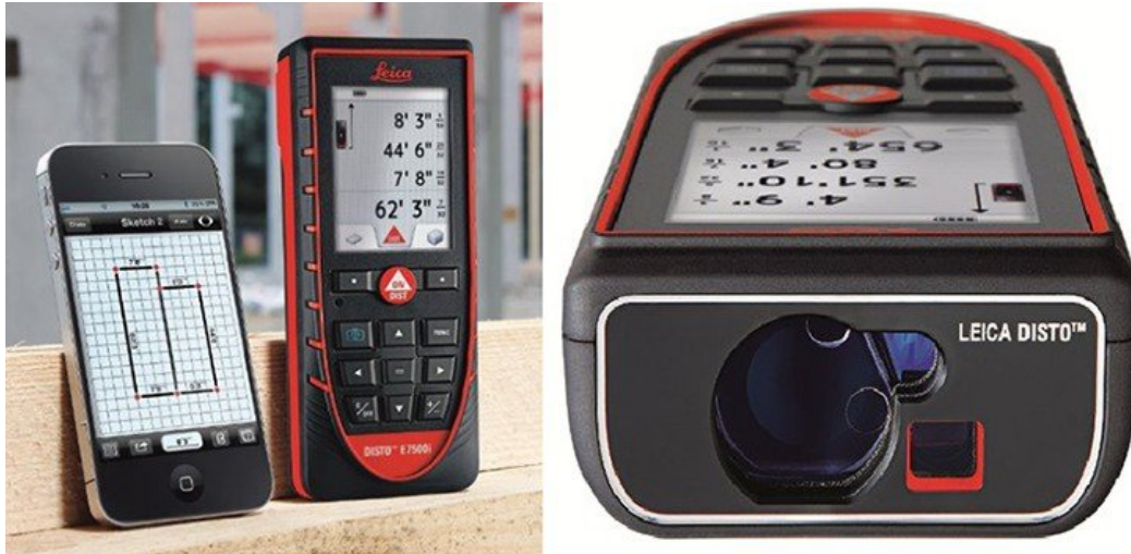
Figure 1: Example Leica DISTO E7500i 660ft Laser Distance Measurer w/Sketch iPad iPhone App
