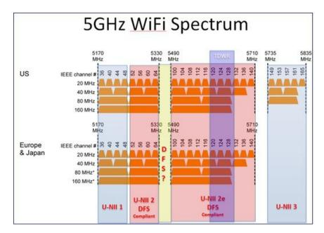
In the US, there are currently 22/10/5/1 channels with bandwidth 20/40/80/160 MHz channels respectively. With the proposed opening up of 5.35 - 5.47 GHz and 5.85 - 5.925 GHz spectrum, the number of channels increases to 34/16/8/3. If the industry manages to take back the TDWR channels, the number of channels increases to 37/18/9/4.
