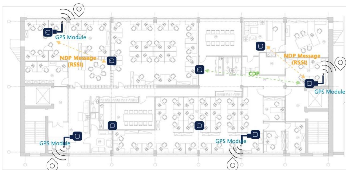
Figure 2. Geolocation Propagation Operation across an Indoor Floor plan
