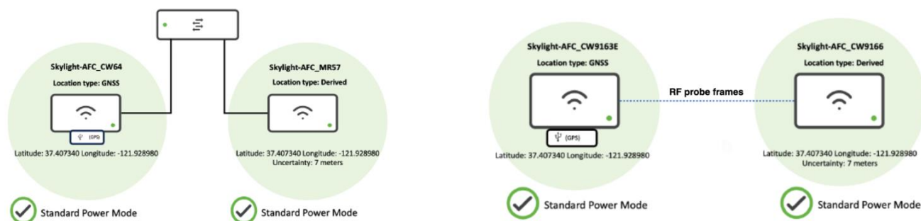
Figure 1. Wired and Wireless Geolocation Propagation Techniques
