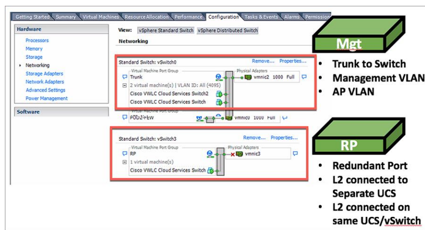
Figure 2. Mapping the hypervisor to the VM management interface in ESXi
