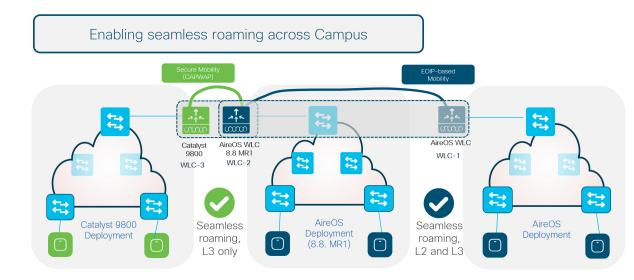
This deployment model uses three controllers running different code versions.
