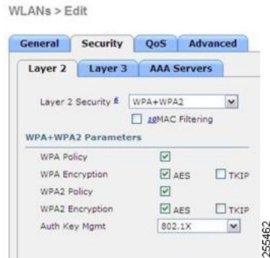
Figure 8: Compatible Security Settings for OEAP Series
