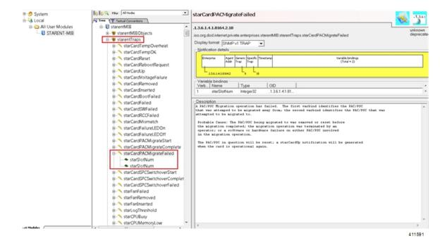
The SNMP MIB browser allows you to search for specific MIBs. You can search for a specific OID (object identifier) to find a specific MIB entry.
