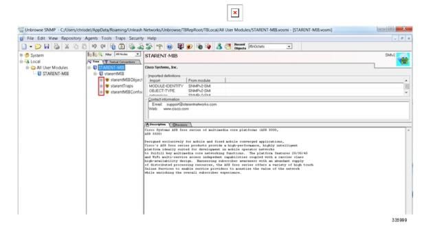
In the example below the MIB Browser presents a tree diagram that allows you to display details for each Object, Trap and Conformance. The example below includes the OID number and trap details for the starCardPACMigrateFailed trap.
