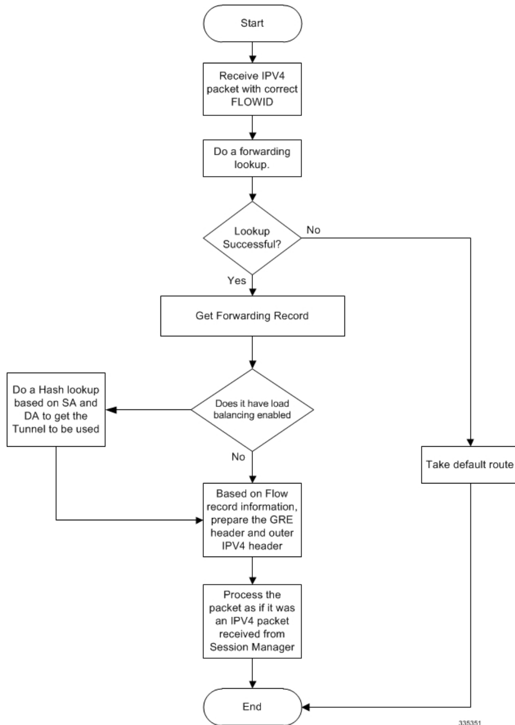
Figure 41: Egress Packet Processing on GRE Interface
