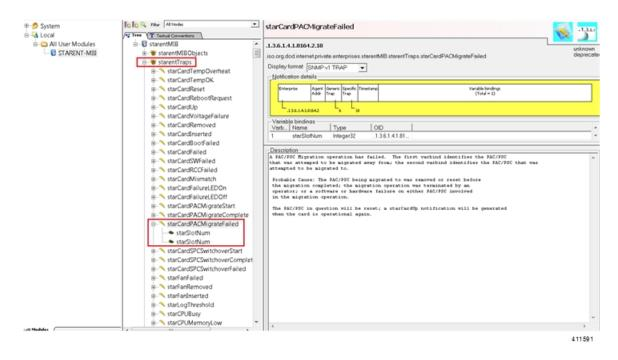
The SNMP MIB browser allows you to search for specific MIBs. You can search for a specific OID (object identifier) to find a specific MIB entry.
