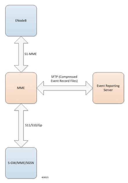
The interface between the MME and the external server is based on SFTP. Each record (CSV record) is generated as comma-separated ASCII values. The MME sends one ASCII formatted CSV record per line. The CSV records are stored in a file. If configured, these files can be compressed before sending it to the external server.
