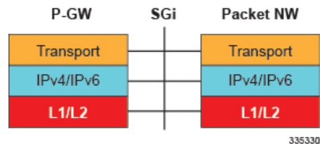
Figure 30: Protocols Supported on the SGi Interface
