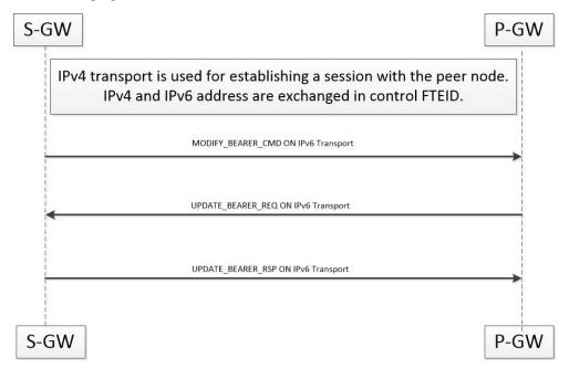
When a session is being established, P-GW, S-GW, and SAEGW node uses the IPv6 address as transport. This transport is used for establishing tunnel with peer node. If IPv4 and IPv6 addresses are exchanged in control FTEID then the node should handle MBCmd, BRCmd, and DBCmd messages on IPv4 transport by the nodes.
