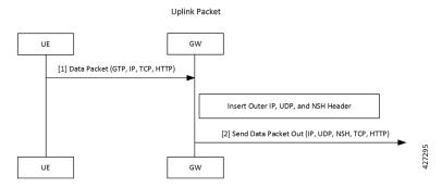
For an uplink packet, if the call flow matches the specified criteria, PGW or SAEGW adds the NSH header to the data packet. NSH header may have variable length context header, which can be encrypted if specified in the configuration.
