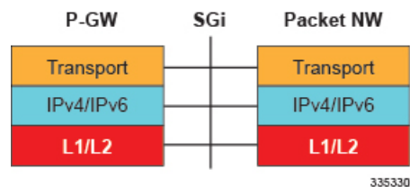
Figure 31: Protocols Supported on the SGi Interface
