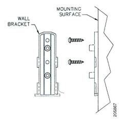
Step 5 Slide the mounting bracket onto the wall bracket and secure it in place (optional) with the two screws provided (Figure 4).
