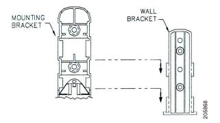
Step 6 To adjust the azimuth and elevation, loosen the bolt that attaches the antenna bracket to the mounting bracket (Figure 5). Azimuth can be adjusted  $\pm 90$  degrees. Elevation can be adjusted  $\pm 15$  degrees and  $\pm 35$  degrees.
