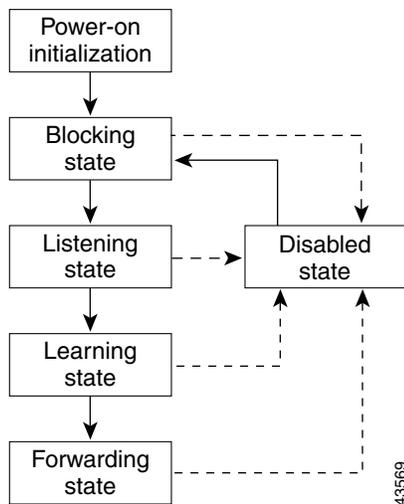
When you enable STP on the access point, the Ethernet and radio interfaces go through the blocking state and the transitory states of listening and learning. Spanning tree stabilizes each interface at the forwarding or blocking state.
