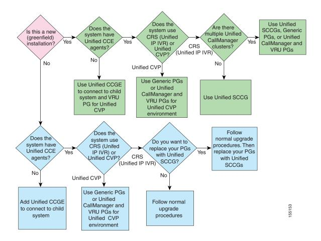
For detailed installation and upgrade information on the Unified SCCG and Unified CCGE, see *Cisco IPCC Gateway Deployment Guide ICM/IPCC Enterprise Edition Release* 7.0(0) at:
