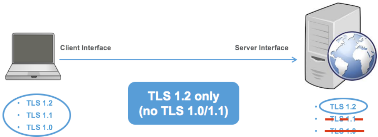
Figure 4: Configuration to Disable TLS 1.0/1.1 Applies to Server Interface
