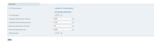
**Credentials refresh interval** specifies the lifetime of the authentication token issued by the Expressway to a successfully authenticated client. A client that successfully authenticates should request a refresh before this token expires, or it will need to re-authenticate. The default is 480 minutes (8 hours).
