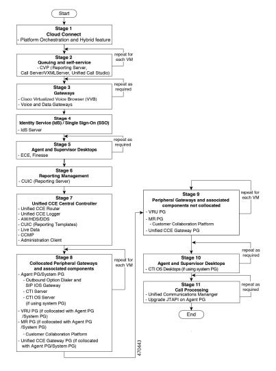
The following diagrams illustrate the stages of the component-level upgrade flows for the Packaged CCE 4000 Agents and above Deployment solution upgrade. Each diagram covers one of the stages. The letter at the end of each flow indicates the start of the next flow that you are required to perform.
