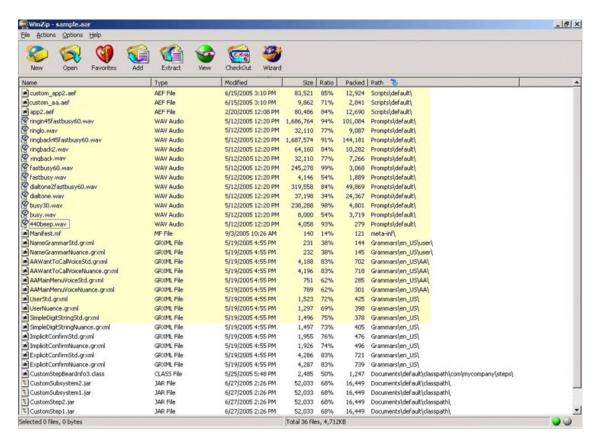
To deploy custom applications, steps, and subsystems through an AAR file, you must first create the AAR file using a jar or zip tool and then upload the file through the Unified CCX Administration web page.
