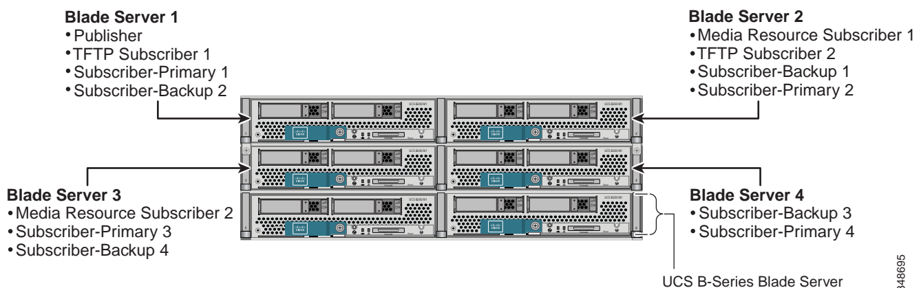
Figure 9-8 Unified CM Server Node Distribution on UCS
