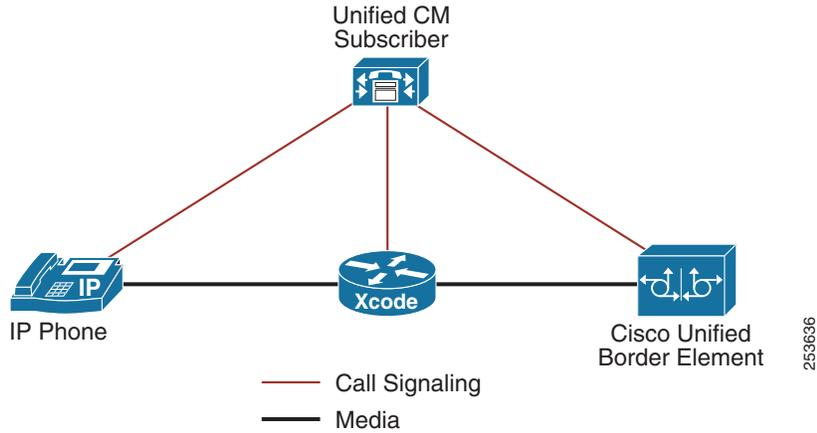
Unified CM communicates with media resources using Skinny Client Control Protocol (SCCP). This messaging is independent of the protocol that might be in use between Unified CM and the communicating entities. Figure 17-2 shows an example of the message flow, but it does not show all of the SCCP or SIP messages exchanged between the entities.
