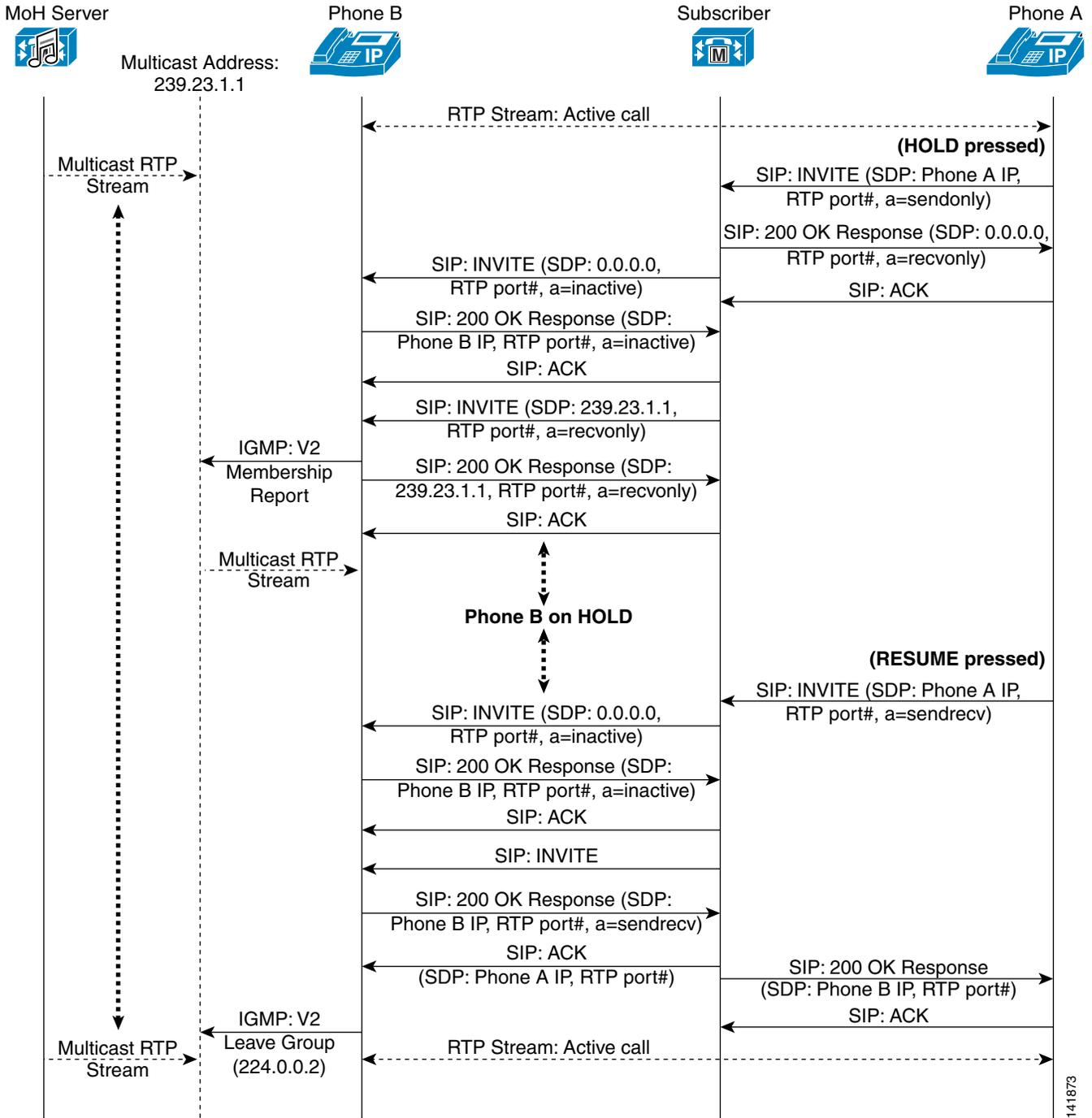
Next, phone B in Figure 17-8 issues an IGMP V2 Membership Report message indicating that it is joining this multicast group. In addition, phone B sends a SIP 200 OK Response back to Unified CM indicating an SDP media attribute of recvonly in response to the previous SIP INVITE. Meanwhile, the MoH server has been sourcing RTP audio to this MoH multicast group address and, upon joining the multicast group, phone B begins receiving the one-way MoH stream.
