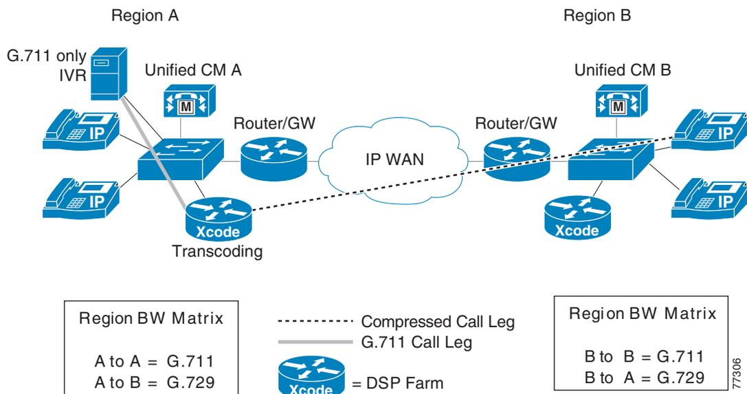
Unified CM uses media resource groups (MRGs) to enable sharing of MTP and transcoding resources among the Unified CM servers within a cluster. In addition, for calls across intercluster trunks, MTP and transcoding resources are used only when needed, thus eliminating the need to configure the MTP service for applications that do not support LBR codecs.
