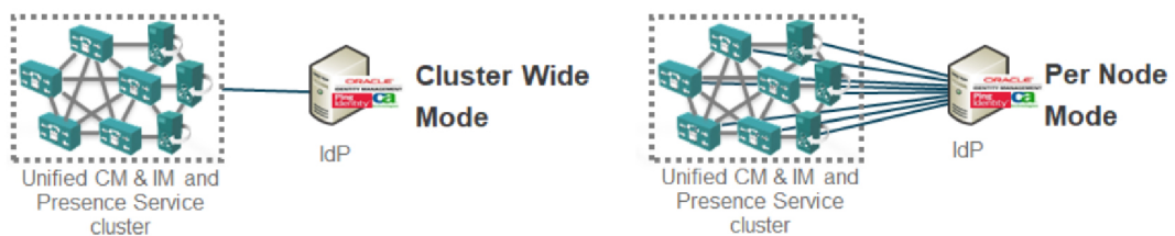
Figure 2: Two types of SAML metadata agreements in Cisco Unified Communications Manager
