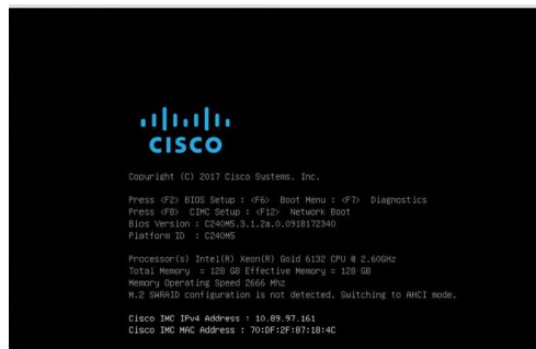
Figure 1: Press F8 at the CIMC Boot Screen
