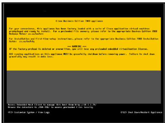
Figure 3: Console Screen After ESXi Loads
