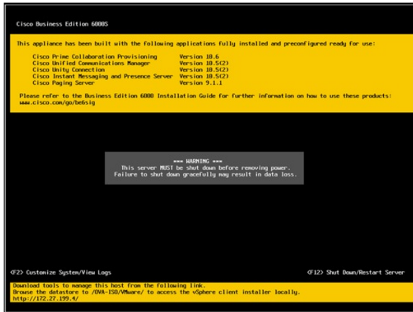
Figure 3: Console Screen After ESXi Loads
