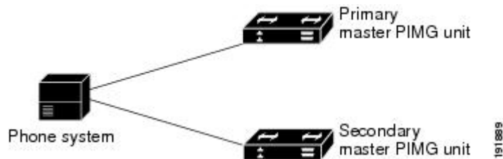
Figure 7: Figure A-7 Serial Cable Connections from Multiple Serial Ports on the Phone System to the Serial Ports on the Master PIMG Units
