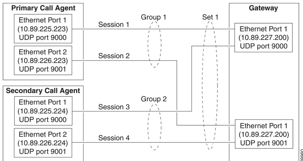
**Step 3** Configure PRI FAS. [Figure 1-6](#) shows a sample configuration for Facility Associated Signaling (FAS).
