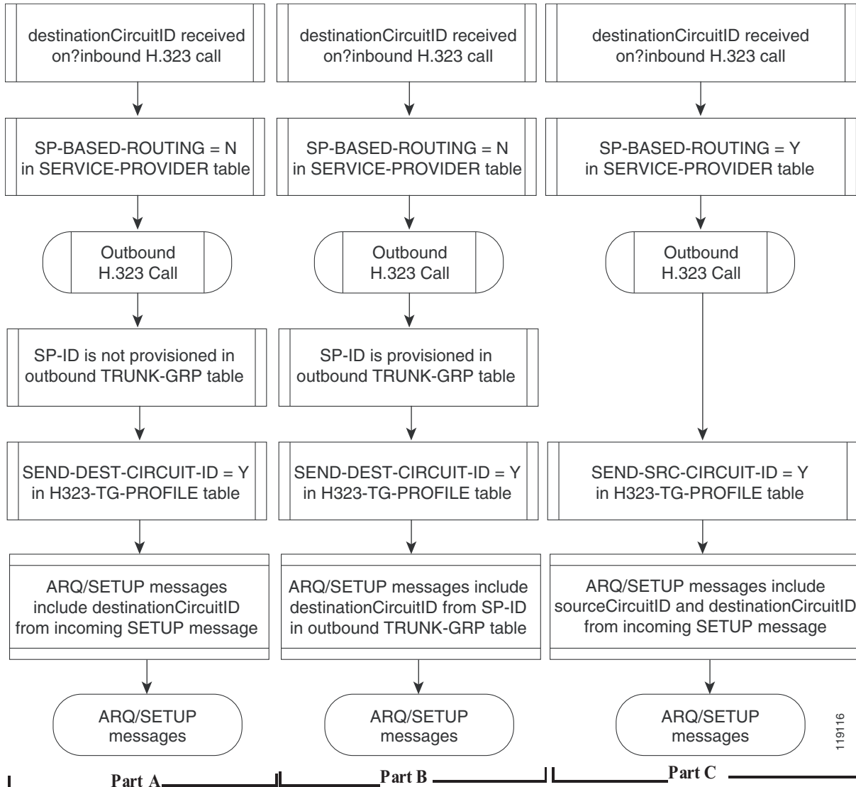
Figure 3-2 H.323 Tandem Calls with Circuit Information Sent
