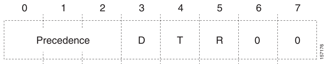
Figure 3-2 TOS Field in the IP Header
