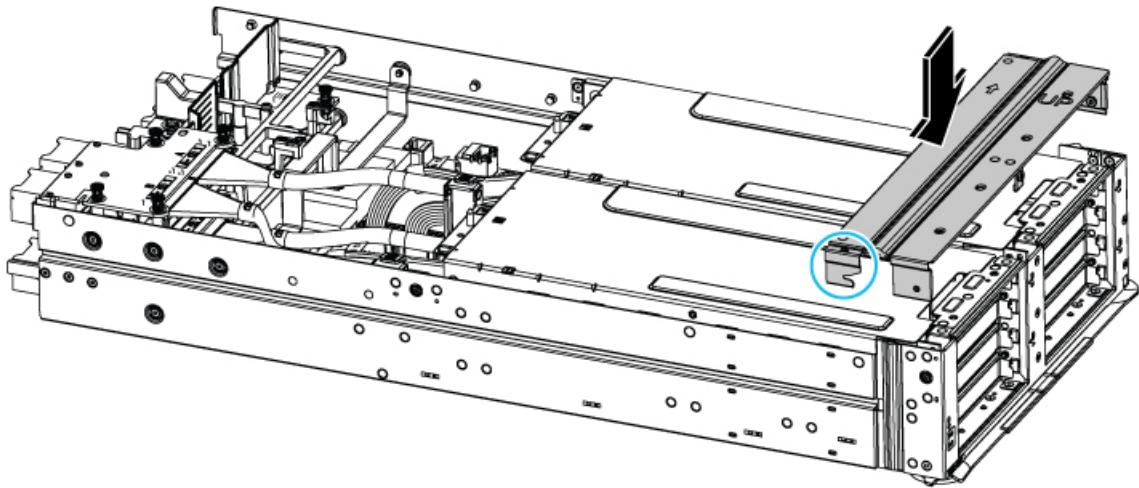
**Step 2** Connect the PCIe node.
