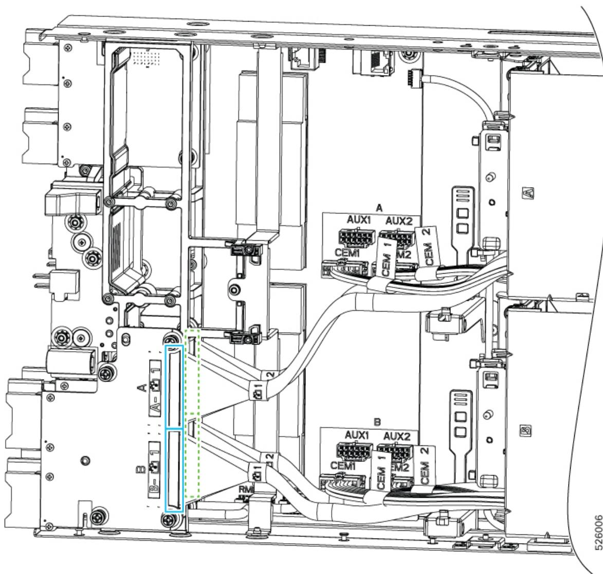
d) Disconnect the power cables from the node's CEM1 and CEM2 motherboard connectors.
