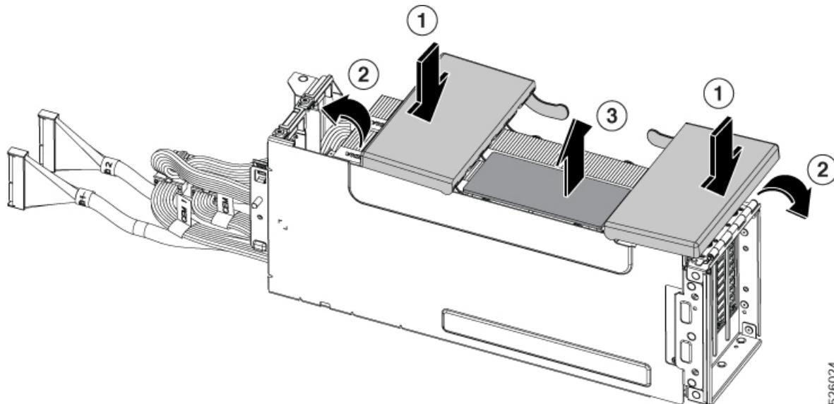
**Step 5** When the GPU interconnect disconnects from the GPUs, grasp it and lift it straight up to remove it.
