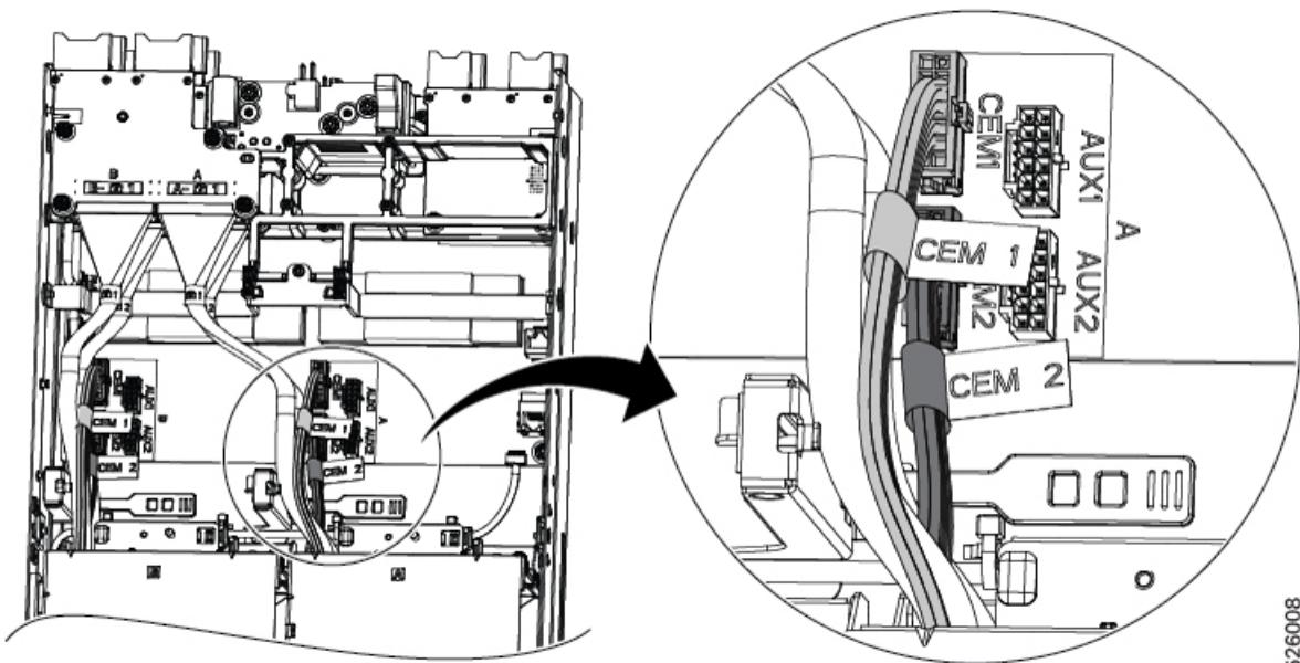
f) Connect the AUX cables to the AUX1 and AUX2 connectors on the node motherboard.
