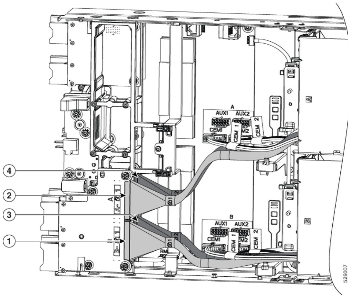
e) Connect the power cables to the node's CEM1 and CEM2 motherboard connectors.
