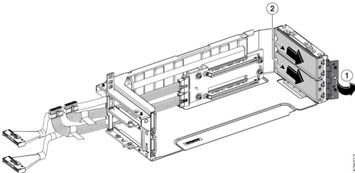
**Step 7** Grasp the GPU, and holding it level, pull it out so that it disconnects from the PCIe socket.
