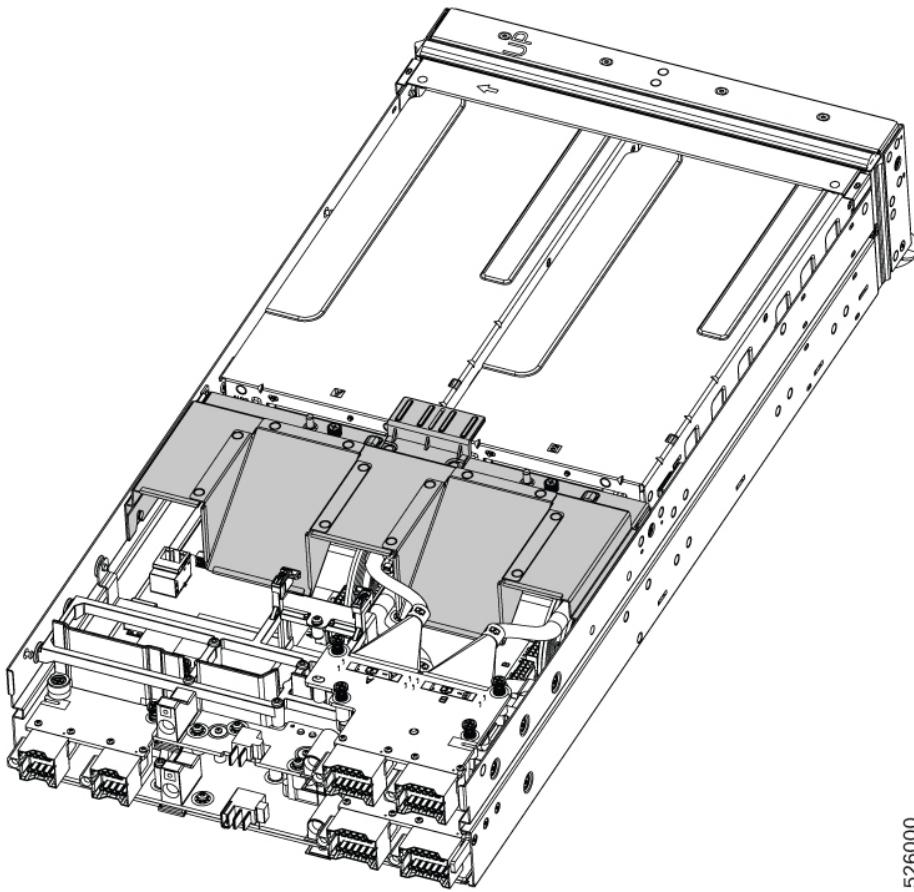
The node's air baffle optimizes the airflow from the cold aisle in the datacenter, across the node's components, and exhausts heated air into the hot aisle of the datacenter. When the PCIe node is operating, the air baffle must be installed and the node's top cover must be installed.
