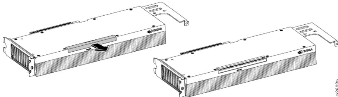
**Step 3** Position the two-way GPU interconnect over the GPUs' connectors.
