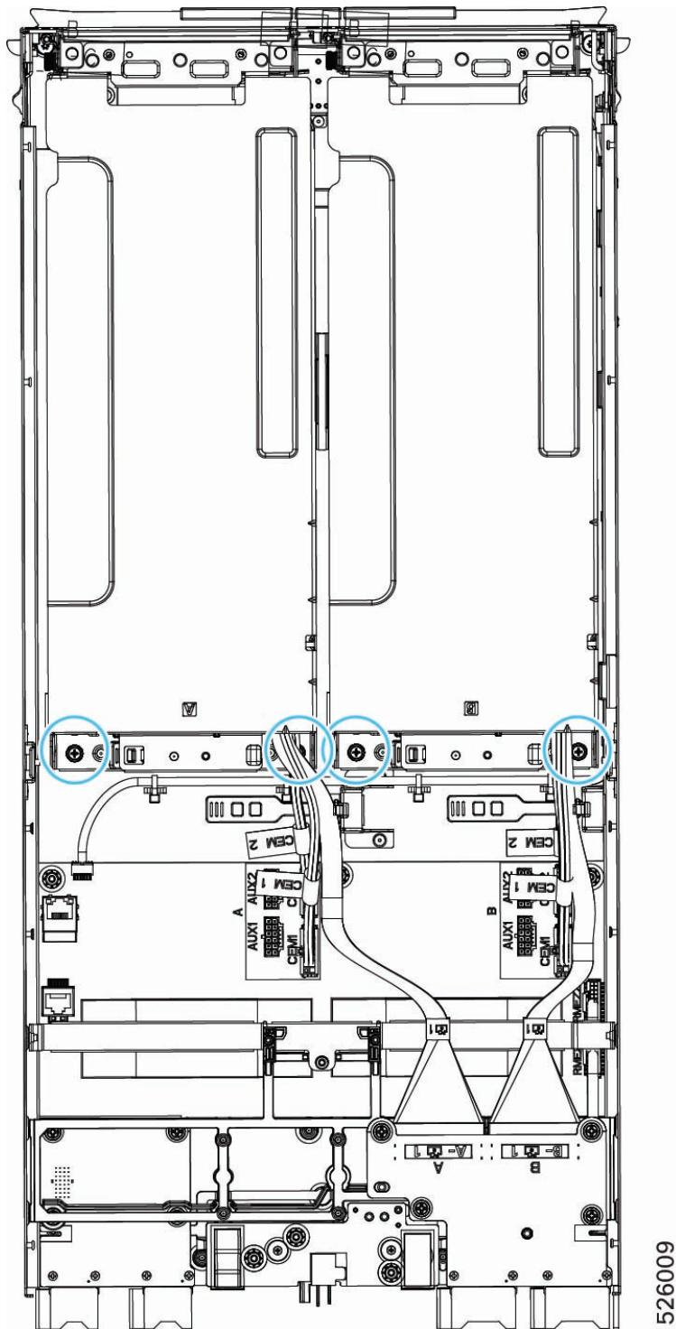
d) Connect the MCIO cables to the rear mezzanine (MEZZ) connector.
