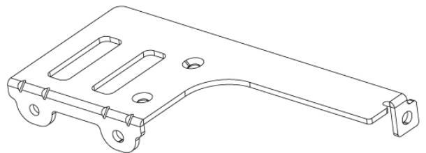
You must replace the legacy extender bracket with the Cisco enhanced extender bracket. Bracket replacement must be completed before installing, or reinstalling, the H200 NVL GPU. For more information, see [Replacing a Legacy GPU Extender Bracket, on page 27](#)
