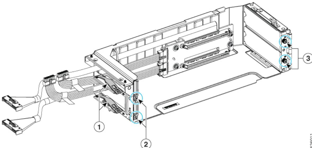
**Step 6** When the Phillips-head screws are loosened, swing the hinged door open so that the GPU can slide out of the slot (1).
