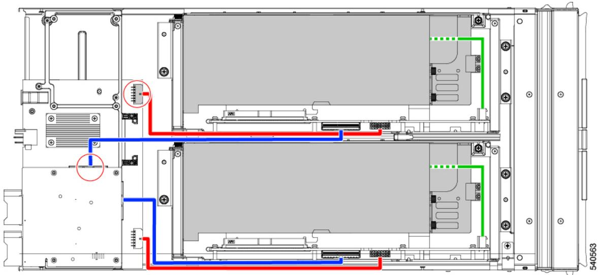
Figure 4: PCB Cable Connectors, HHL GPU
