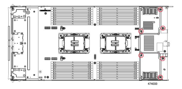
**Step 6** Using a T10 screwdriver, remove the two standoffs next to CPU 1, which is nearest to the front of the compute node.
