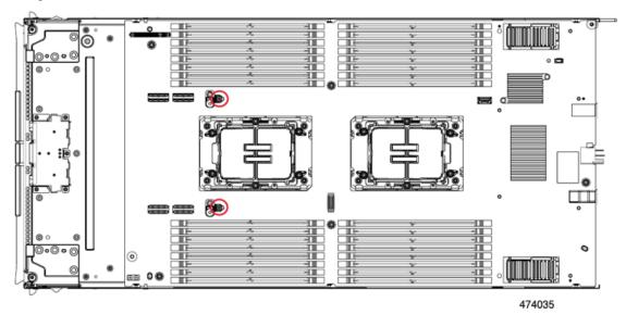
**Step 7** Using a T10 screwdriver, remove the Torx screws that secure the primary PCB to the midframe.
