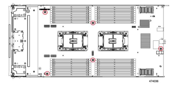
**Step 8** Using a T20 screwdriver, loosen the captive Torx nuts that hold each CPU bolster plate, then remove the plates. There are six nuts for each plate.
