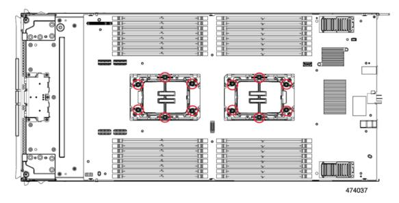
**Step 9** Grasp the primary PCB along the edges and lift it up to disconnect it.
