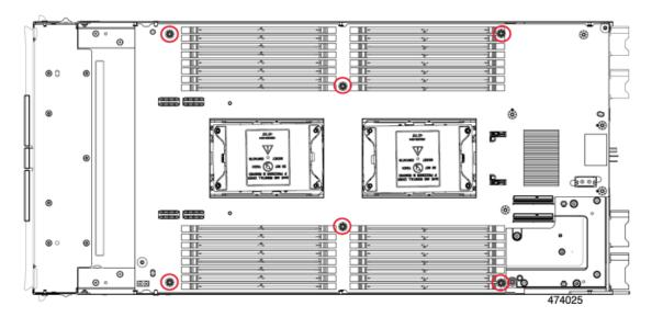
**Step 10** Using a T20 screwdriver, loosen the captive Torx nuts that hold each CPU bolster plate, then remove the plates.
