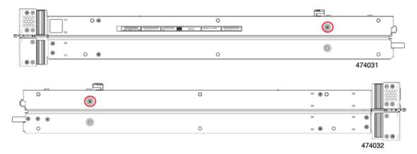
**Step 5** Using a T10 screwdriver, remove the Torx nuts from the top of the rear mezzanine frame, then remove the primary's rear mezzanine frame.
