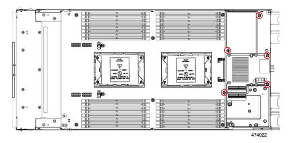
**Step 8** Using a T10 screwdriver, remove the two standoffs next to CPU 3, which is nearest to the front of the compute node.
