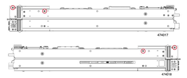
b) When all four screws are removed, lift the secondary front mezzanine module to disconnect it from the motherboard.
