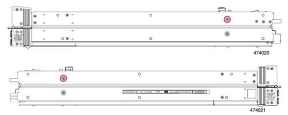
Step 7 Using a T10 screwdriver, remove the Torx nuts from the top of the rear mezzanine frame, then remove the rear mezzanine frame.
