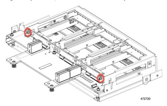
b) Grasp the drive backplane and lift it off of the sheetmetal frame.
