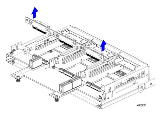
**Step 3** Disconnect the PCBA from the sheetmetal frame.
