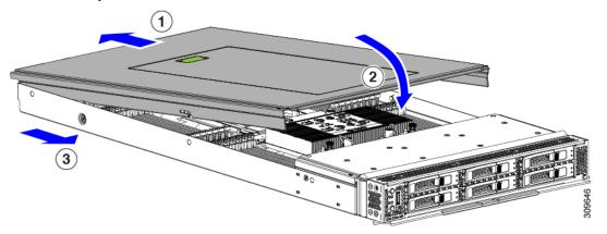
**Step 3** Keeping the compute node's cover flat, slide it forward until the release button clicks.
