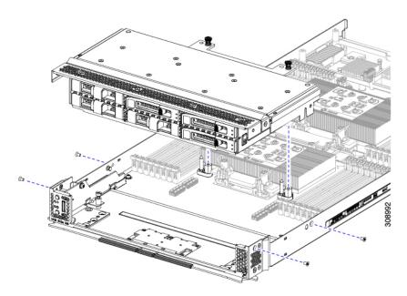
**Step 3** Making sure that all the screws are removed, lift the front mezzanine module to remove it from the compute node.
