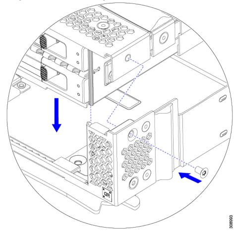
b) Using a T8 screwdriver, insert and tighten the four screws, two on each side of the sever node.
