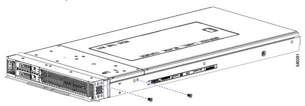
**Step 6** Replace the compute node top cover and reinstall the compute node into the chassis.
