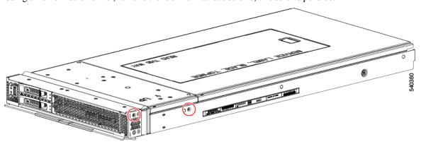
b) Using a #2 Phillips screwdriver, loosen the two #2 Phillips captive screws at the rear of the front mezzanine module.
