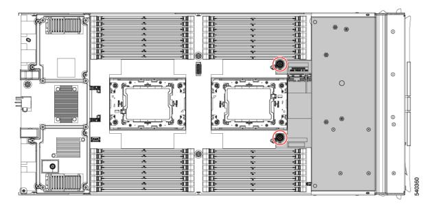
Step 3 Grasp the front mezzanine module at the middle of the top front edge and lift the front mezzanine module straight up to remove it from the compute node.
