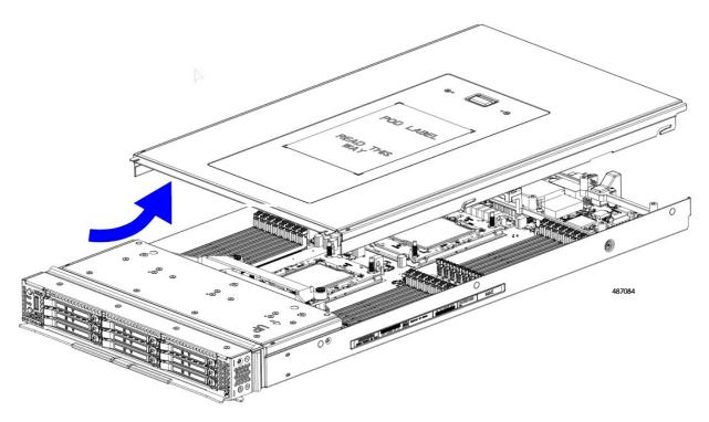
**Step 2** While holding the back end of the cover, slide it back, then pull it up to lift the top cover off of the compute node. By sliding the cover back, you enable the front edge to clear the metal lip on the rear of the front mezzanine module.
