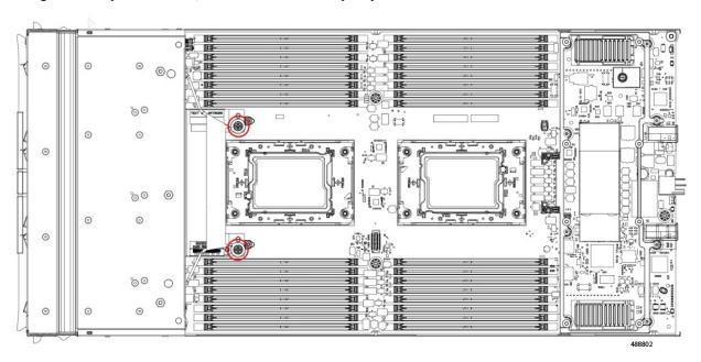
Step 3 Grasp the front mezzanine module at the middle of the top front edge and lift the front mezzanine module straight up to remove it from the compute node.
