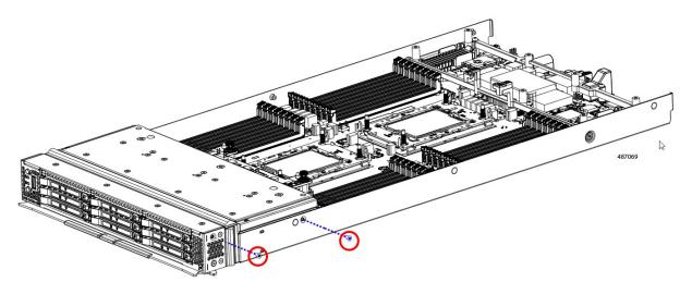
**Step 6** Replace the compute node top cover and reinstall the compute node into the chassis. See Installing a Compute Node Cover, on page 2.
